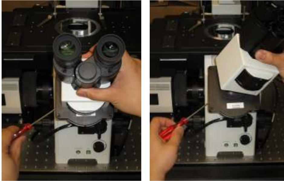
**Removing the Eyepiece**
