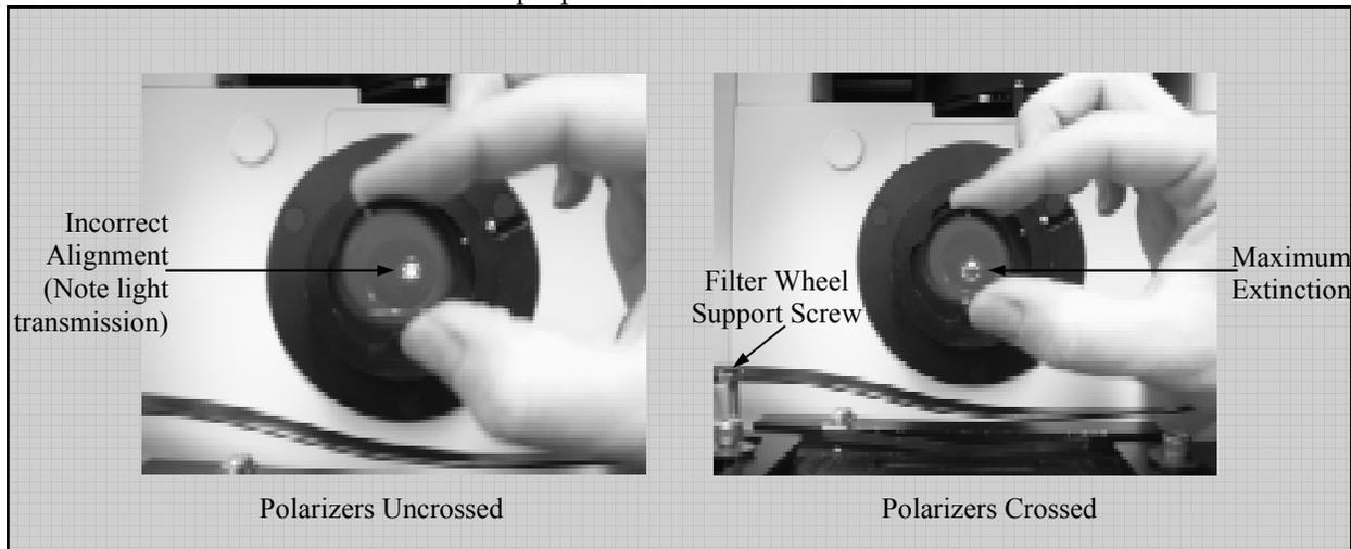
Figure 4. Proper Polarizer alignment.
