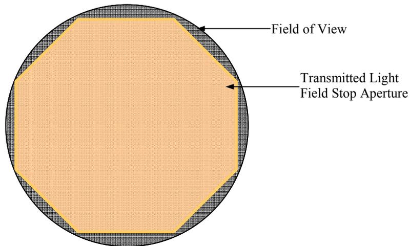
*Figure 3. Köhler Illumination Alignment for the Transmitted Light.*
