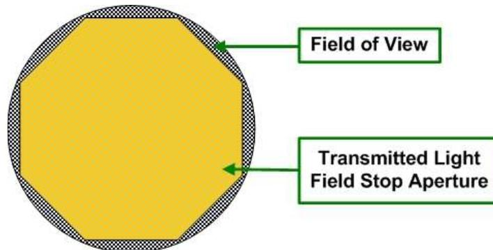
If you cannot see the entire iris while moving the Condenser Focus Knob, it may be necessary to alter the centering before you are able focus on the edges of the iris.
