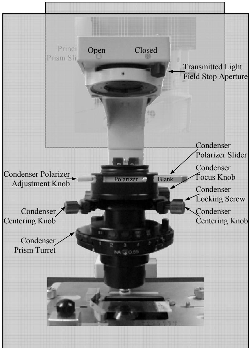
Figure 1. DIC Condenser Assembly.
