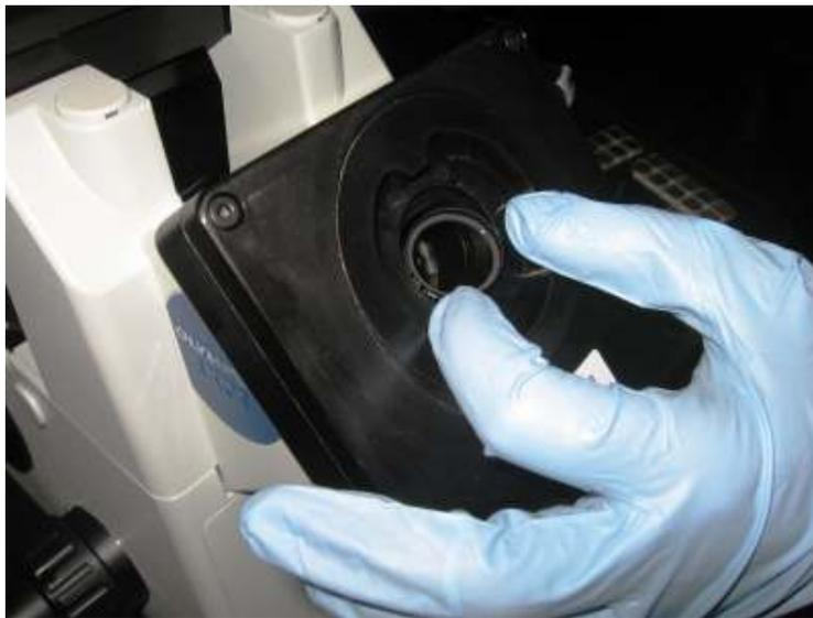
**Removing the Polarizer from the Eyepiece Filter Wheel**
