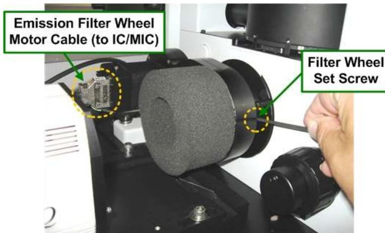
**Removing the Emission Filter Wheel**
